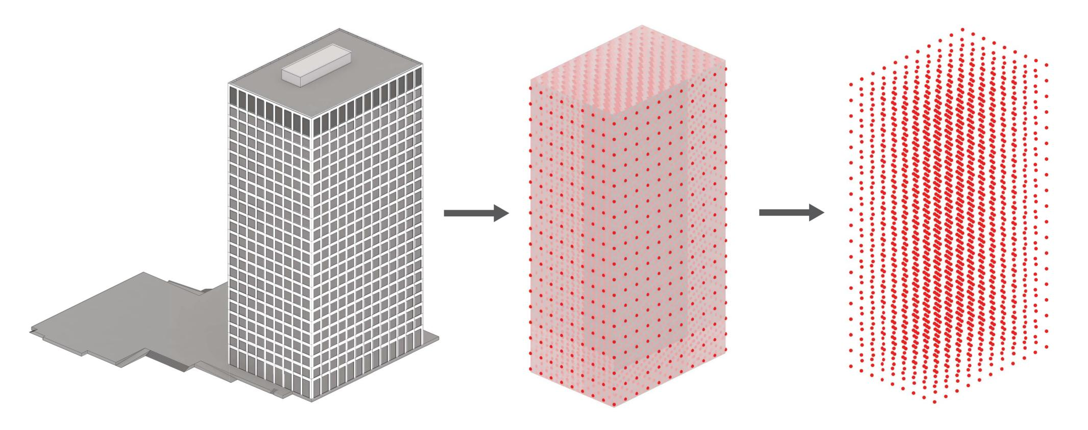
NOTE : POINT CLOUD DENSITY IS ADJUSTABLE BASED ON FUNCTIONAL NEEDS AS PER CITY PLAN (POINT CLOUD FROM RHINO MODEL EXTRACTED TO GRASSHOPPER)
